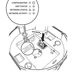
No DIP switch settings are required for the system. Before installing the dome drive verify that switch SW1-1 (SW1, switch 1) is set to the ON position and all other switches are set to the OFF position.
